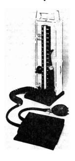
The zero-muddling manometer is only slightly larger than the conventional sphygmomanometer and operates in the same way, except that a wheel is spun before each measurement to adjust the zero to an unknown level. Once the blood pressure has been measured the level of zero may be determined and the pressure reading corrected.
